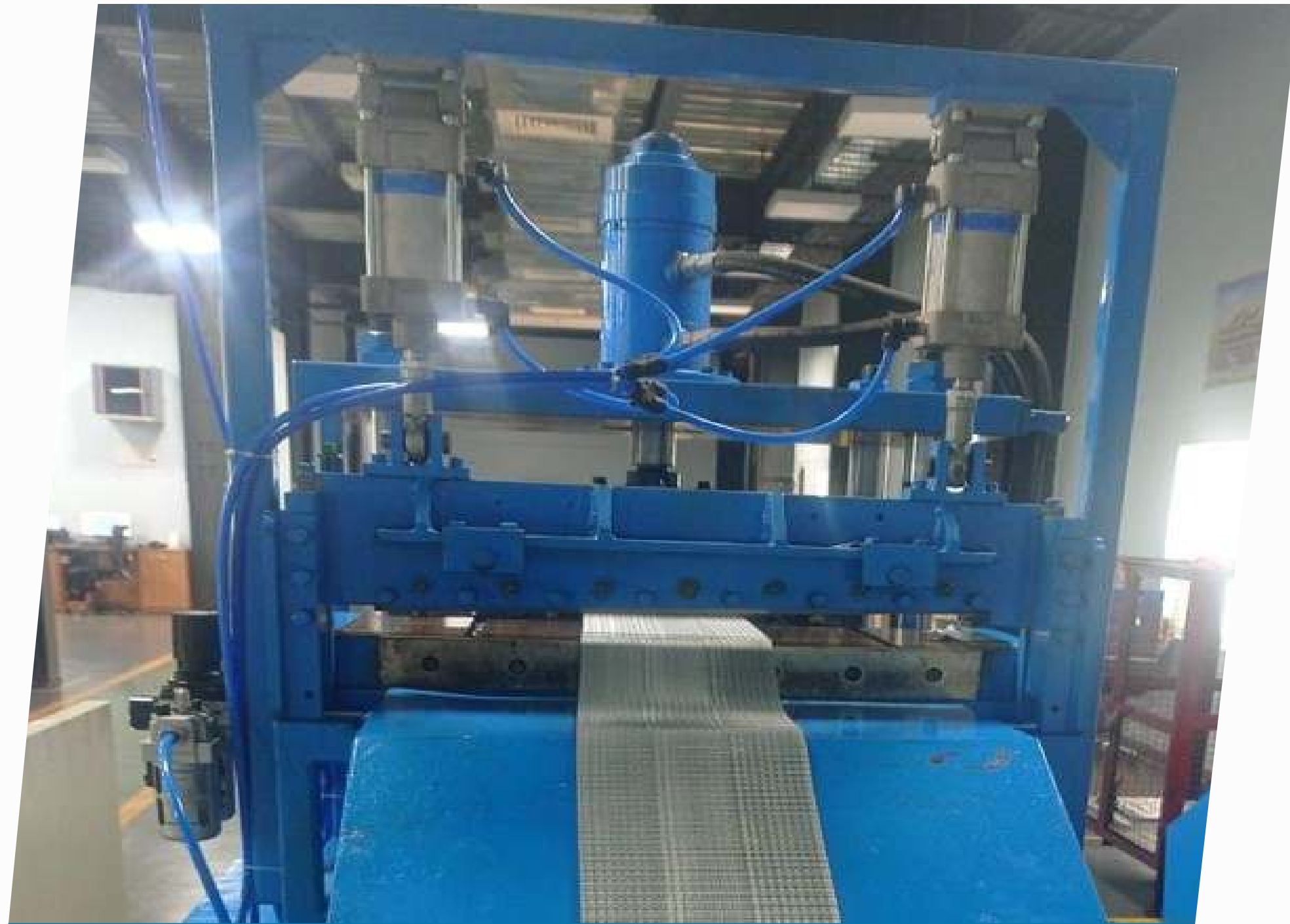
Corrugated Fin Manufacturing Machine
